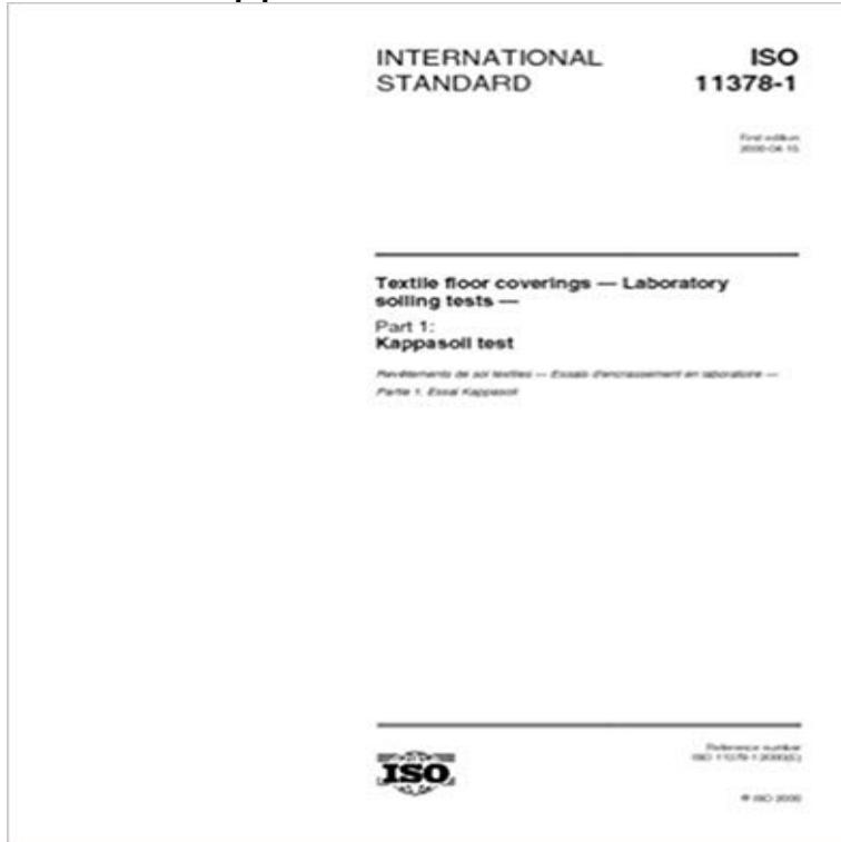
This part of ISO 11378 specifies a method for assessing the propensity of textile floor coverings to soiling using an artificial soil composition. The scope of this test method can be extended to assess the efficiency of cleaning chemicals, and cleaning equipment (see annex A). This title may contain less than 24 pages of technical content.
